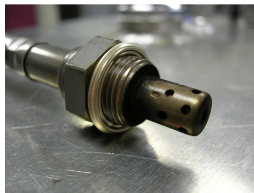
Figure 3.5. Horiba Mexa-700 \lambda display and sensor
