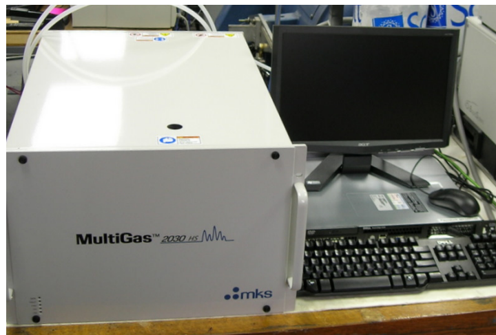
Figure 3.7. MKS Multi-Gas 2030 FTIR exhaust gas analyzer
