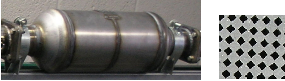
Figure 3.15. Diesel particulate filter and inside catalyst
